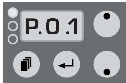
Adjusting of the wait time in minutes (0.1-99)
