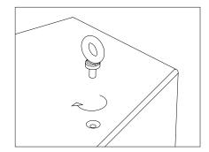
**NOTE:** The rigging points are designed to suspend single enclosures only. There is no facility to hang an additional cabinet below a flown TL series enclosure.
